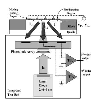
Figure 4. The schematic of the setup integrating the directional microphone diaphragm with optical sensing circuitry. This hand-held setup (10cm×10cm×25cm) is used for both dynamic characterization using electrostatic actuation and also acoustic characterization in anechoic chamber.
