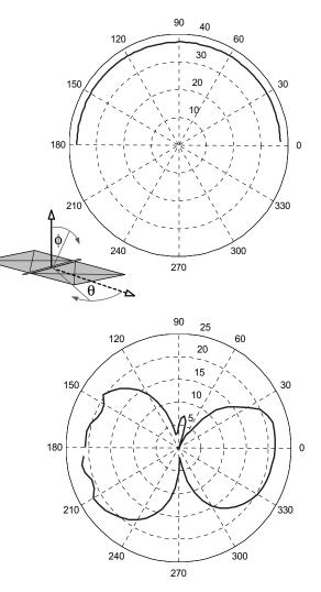
Figure 5. Variation of acoustic response (in dB) of the microphone measured at 2 kHz. Top: Device response in the  $\varphi$  direction showing expected omnidirectional behavior. Bottom: Variation of device response in the  $\theta$  direction showing expected figure-8 behavior.
