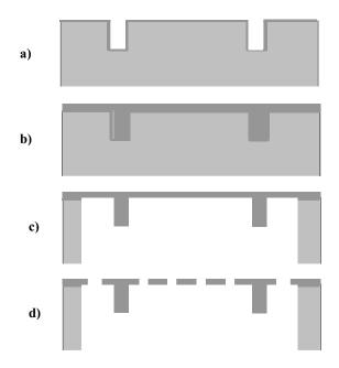
Figure 2. Fabrication process flow for the differential microphone diaphragm with inter-digited fingers at the ends. a) Deep RIE and thermal oxide growth. b) Polysilicon deposition and chemical mechanical polish. c) Backside RIE and thermal oxide removal. d) Polysilicon RIE for fingers and slits.
