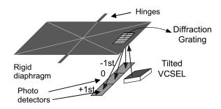
Figure 1. Schematic of a micromachined direction microphone with integrated optical readout.
